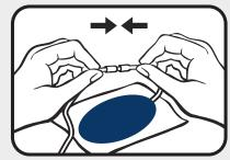
While disconnecting or inserting pin, hold the pin connector
