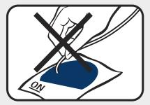
Do not remove Electrodes by pulling the leadwire.
