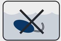
Do not submerge Electrodes in water.
