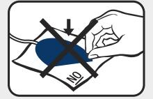
Do not place Electrodes on the «NO» side of the Release Liner.
