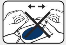
Do not pull the leadwire to remove the pin.
